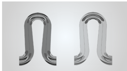
Figure 4.2.1.: Meridional stress on a double-wall metal bellows at axial tensile (left) and at external compressive load (right)
