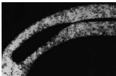
Figure 18.6 Crevice corrosion on a cold strip made from austenitic steel. Sectional view (50-fold enlargement).
